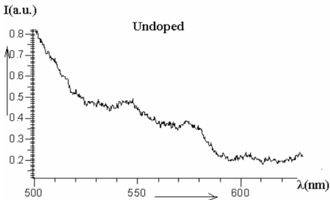
Figure 3a: Fluorescence emission spectra of undoped PMMA
