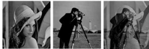
Figure 2.3: Alpha-blending example: (a) first image; (b) second image; (c) blended image using \alpha=0.5
