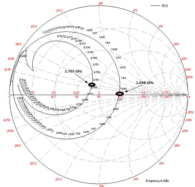
Fig 11 Measured input impedance on a Smith chart for proposed antenna with capacitive loading (C= 1pF)
