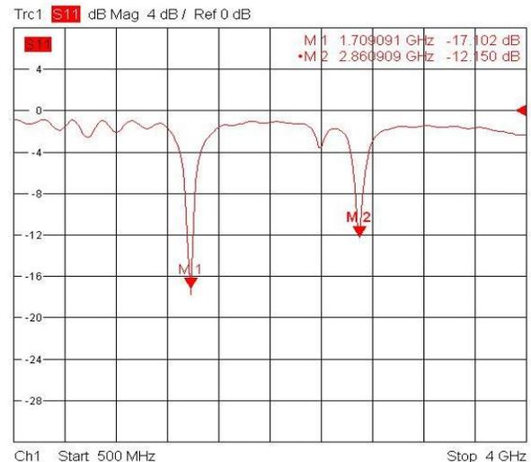
Fig 5 Return loss (dB) v/s frequency (Fabricated Antenna)
