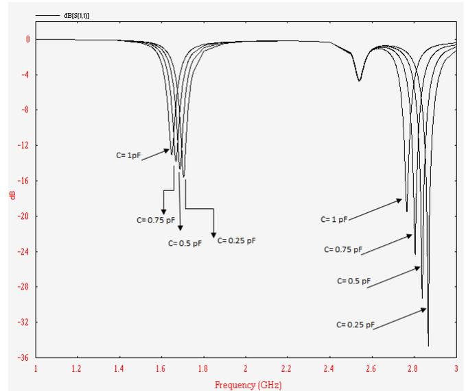
Fig 10 Return loss with varying capacitances
