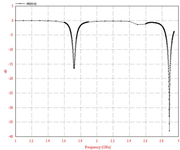
Fig 4 Return loss (dB) v/s frequency (Simulated)
