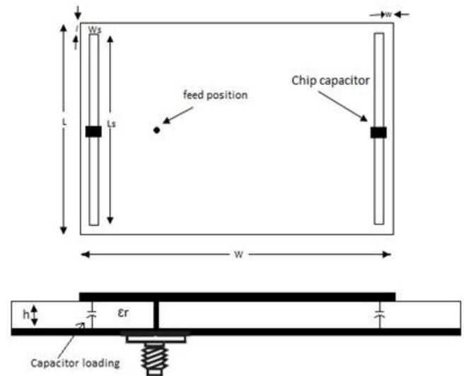
Fig 8- topview & sideview of designed antenna with parallel slots & capacitor loading
