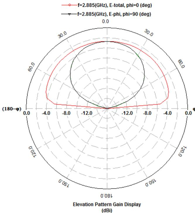
Fig 7 Elevation pattern gain display (dBi) at 2.885 GHz
