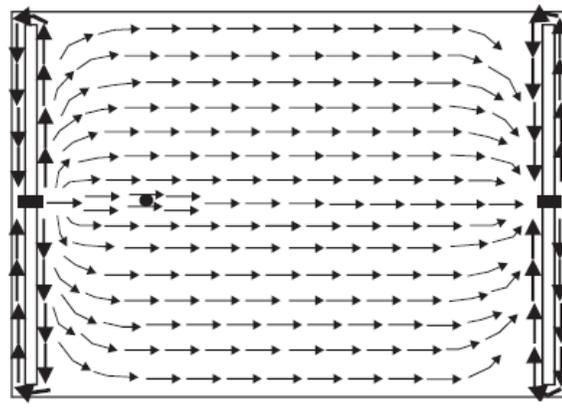
TM300 mode with loading capacitance = 1pF
