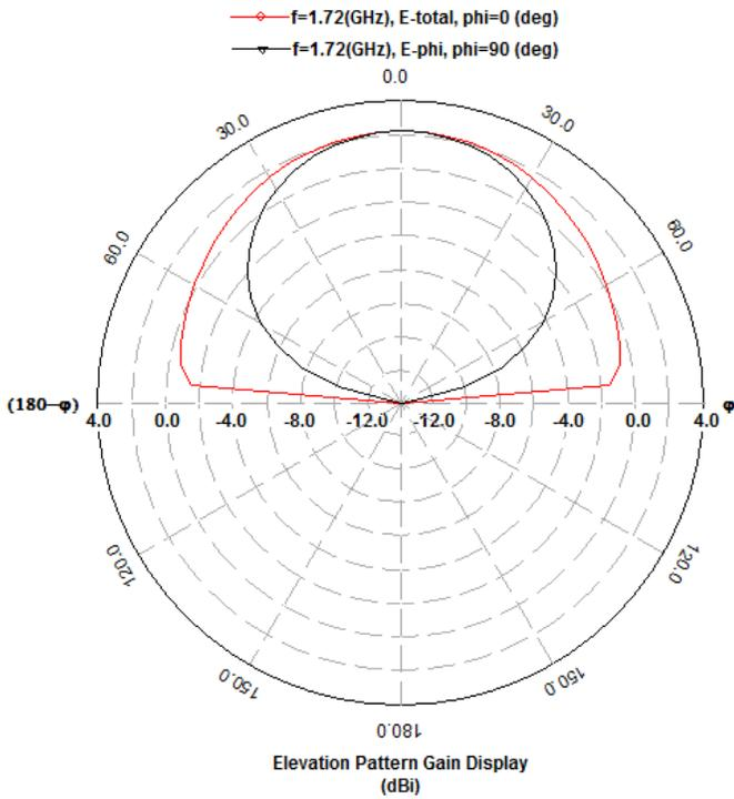
Fig 6 Elevation pattern gain display (dBi) at 1.72 GHz
