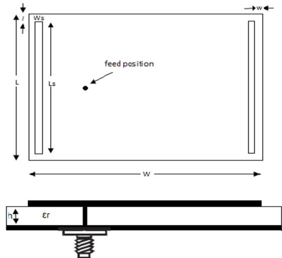
Fig 3 top & side view of designed antenna with parallel slots Authors have c probe feeding.
