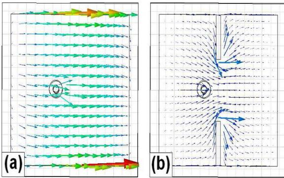
Fig. 2 Current distributions for TM100 mode (a) without slots & (b) with slots.
