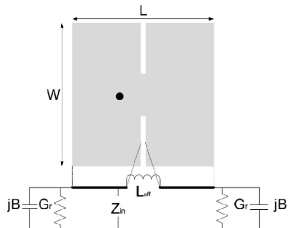
Fig1 Transmission line equivalent
