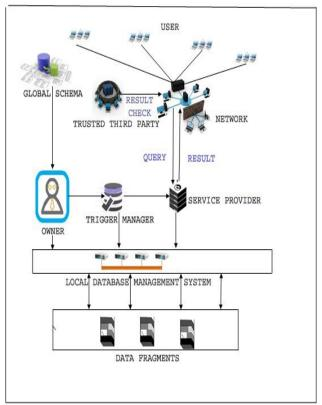
Figure 4: Structure of verification mechanism
