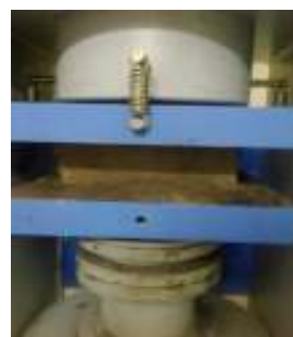
Figure 4.9: Before Failure of Brick
