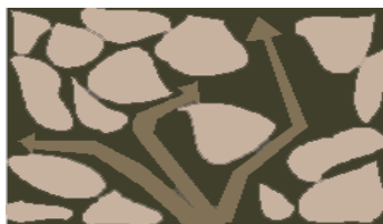
Fig.1 Ability to transmit water
