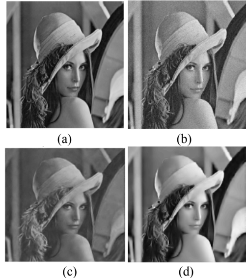
Figure 8: (a) Input Image, (b) Gaussian noisy image for \sigma=10 , (c) Denoised with Dual Tree CWT (d) Denoised images with Double Density DWT
