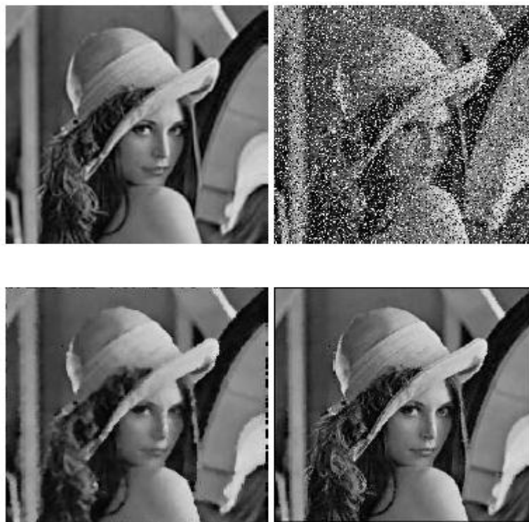
Fig 4 : Results of filtering with a 3X3 median and conditional median filter. From left to right, first row: original Image, noisy image; second row: standard median filter, Adaptive median filter.
