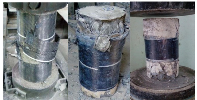
Figure 10. Failure patterns of FRP confined concrete
