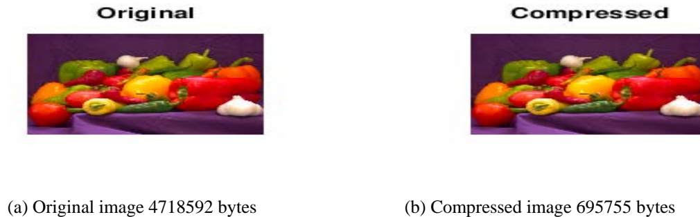
Fig. 2 Examples of image compression technique using JPEG standard
