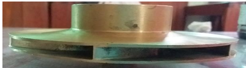
Figure.22. PAT Impeller Bullet Tip Modification
