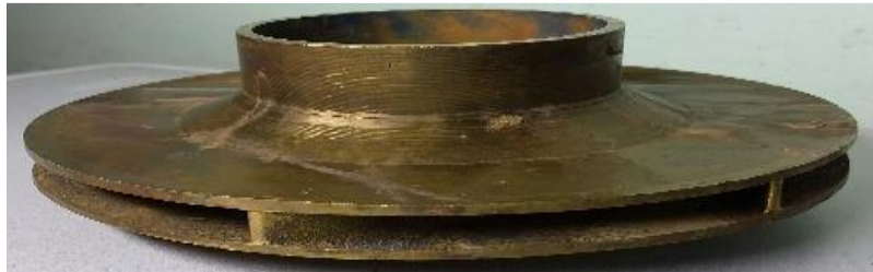
Figure.21. PAT Impeller Round Tip Modification
