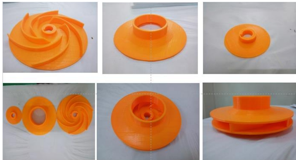
Figure.13. Primary Pattern of Impeller Produced by 3D Printer ( Using PLA Material )
