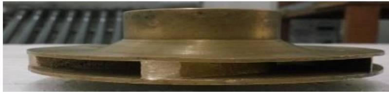
Figure.20. PAT Impeller Sharp-edge Tip Modification
