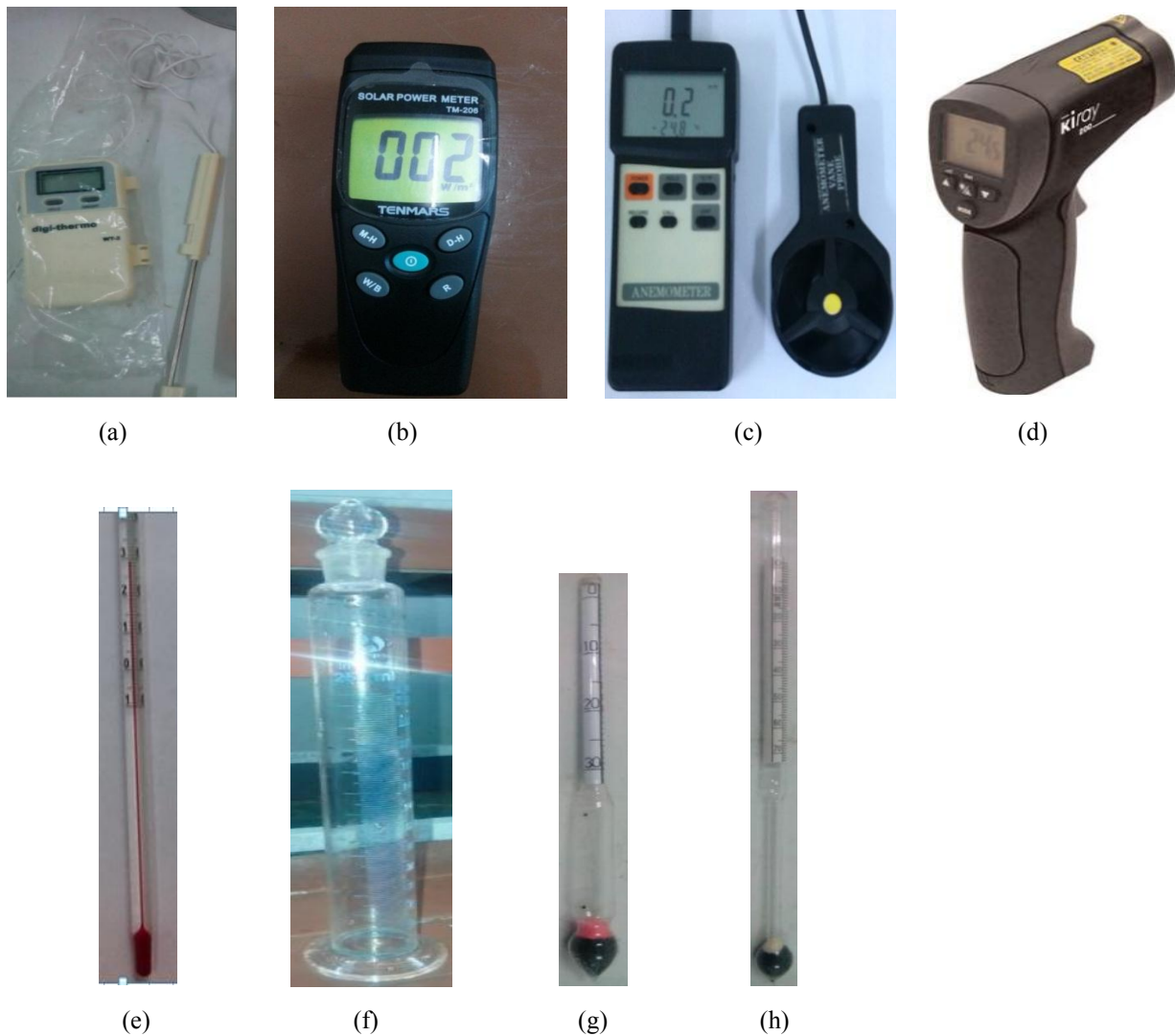
Figure 12. Measuring Instruments (a) Digital Thermometer, (b) Solar Power Meter, (c) Digital Anemometer, (d) Thermometer, (e) Infrared Thermometer, (f) 250 ml Measuring Cylinder, (g) Salt Meter, (h) Hydrometer
