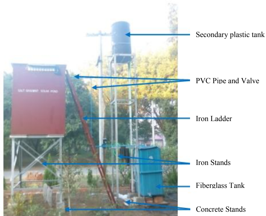
Figure 9. Photographic View of Experimental Set up of Salt Gradient Solar Pond
