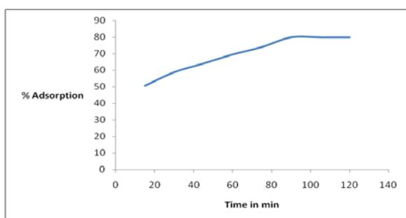
**Fig:4** Effect of contact time on the adsorption of MB on to the adsorbent
