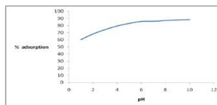
**Fig:1** Effect of pH on the adsorption of MB on to the adsorbent
