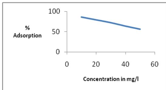
**Fig:3** Effect of dye concentration on the adsorption of MB on to the adsorbent
