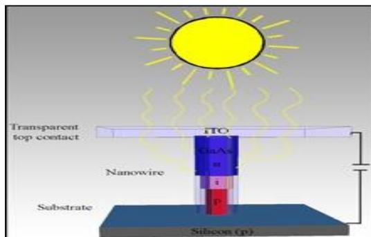
**Fig-2 Nanowire solar cell**
