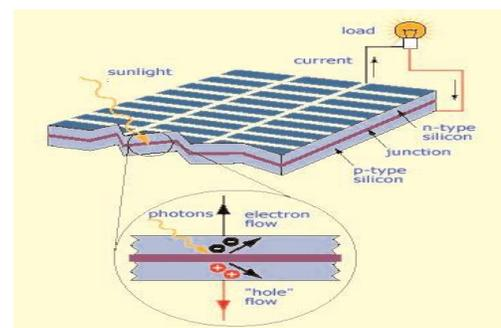
Fig.1 Photovoltaic effect
