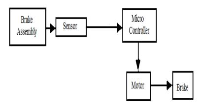
Brake pedal will give analog output voltage when brake is pressed. This voltage value is given as input to the micro controller. Optical sensor is used to detect the speed with which brake pedal is pressed. Optical sensor is placed at 70% of brake pedal path. Optical sensor gives analog value which has to be converted into digital value for analysing. Optical sensor values are given as input to micro controller.
