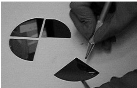
Figure 5: Wafers being cut out into smaller pieces
