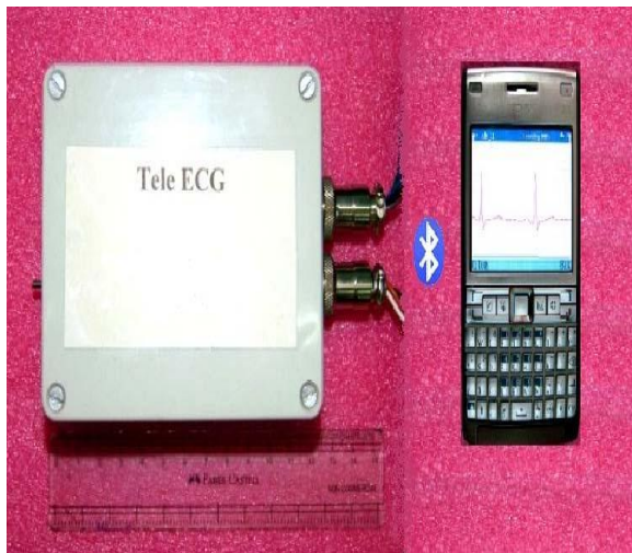
Figure 10: ECG signal received on Mobile Phone
