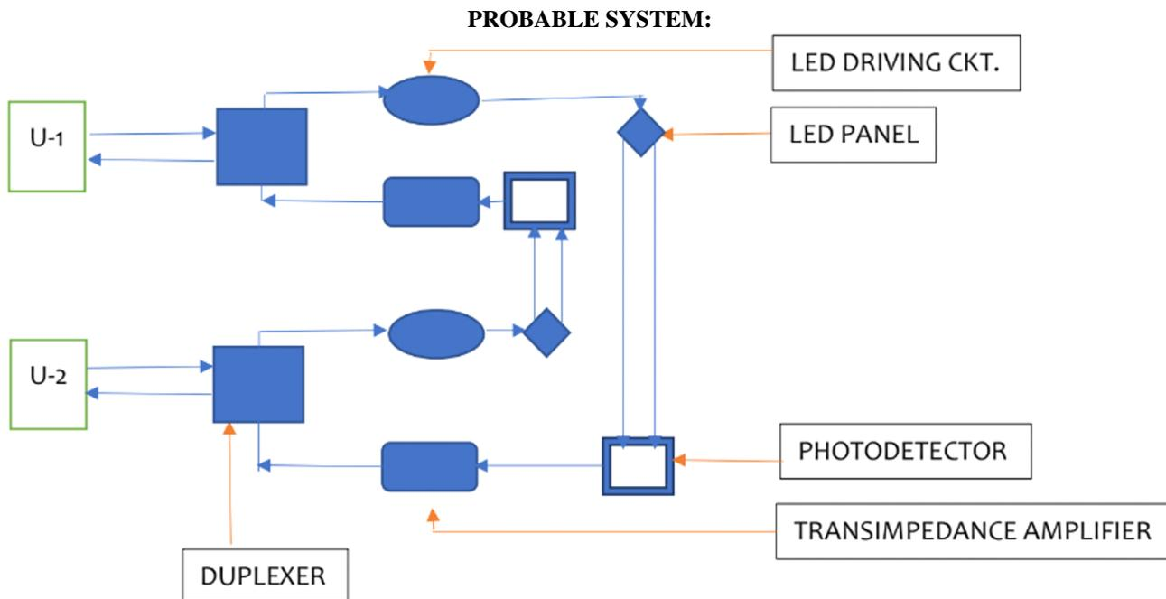
So, the above system provides an underwater communication system. Both the user uses duplexer as it is needed to communicate and receive data at both the sides. The arms have amplifier and led driving circuit each for modulation and receiving purpose respectively.
