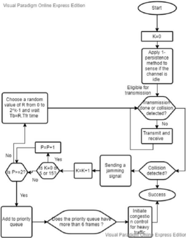
Figure 1: modified CSMA/CD Flowchart with Network Priority Queue
