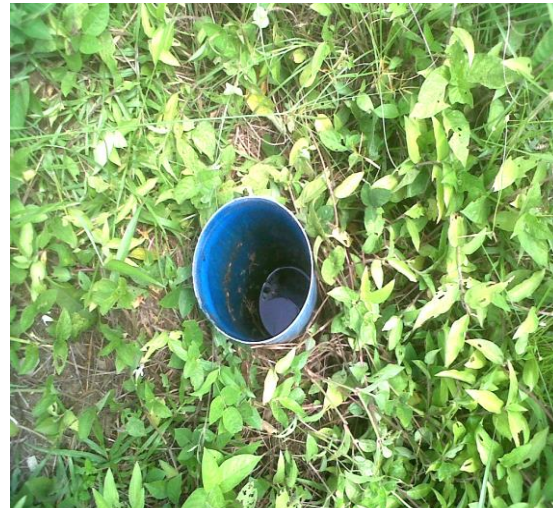
PLATE 2: Perforated PVC pipes used for sampling of leachates from the dumpsite
