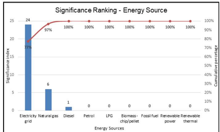
Based on the above analysis, electricity is main source which consuming more energy. Electricity is subdivided again to get more information about which activity or processes use more electricity. The figure below shows significance index for activities, processes and equipments consuming energy.
