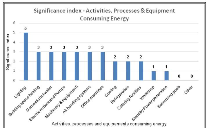
From above figure, it is clear that lighting is main energy consuming activity. There are also few other processes and activities such as domestic hot water, electric pump etc. which are also using more electricity. But, comparing with their investment cost, replacement of motors or development that is more expensive. So, it is better to replace light bulb which is a more reliable option.
