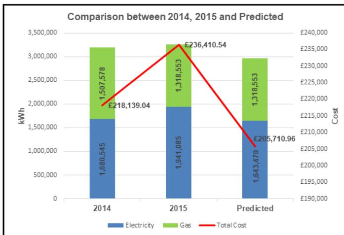
From above calculation, it is clear that if an existing bulb is replaced with LED which gives overall **11.27%** savings over 2014 year.
