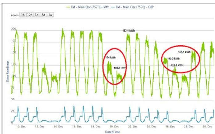
With the help of this profile, it is easy to find out where and when energy is consuming more. By properly monitoring and investigating these energy consumptions, it can be helped to reduce overall consumption.
