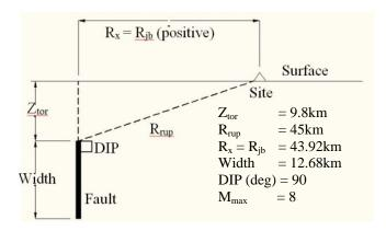
Figure 3: Strike slip faulting system
