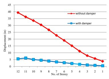
Figure 11 - Displacement diagram of Joint 949
