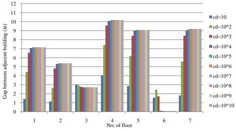
Figure 6 – Gap between adjacent buildings for each floor
