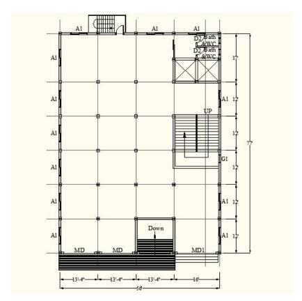
Figure 1: Ground floor plan of 12-storied steel building
