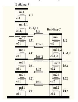
Figure 4- Schematic dynamic model of two adjacent buildings
