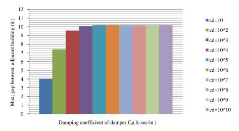
Figure 7 - Max; gap diagram between adjacent buildings for corresponding damping coefficient
