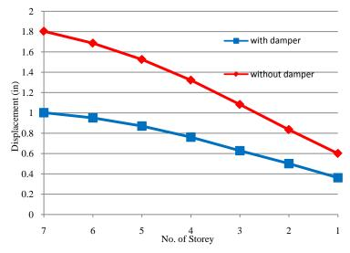
Figure 12- Displacement diagram of Joint 656
