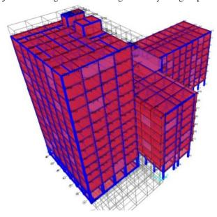
Figure 5 – 3D Model of Adjacent buildings connecting with damper
