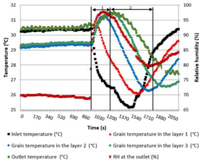
FIGURE 2: The observed rice grain temperature in the three layers, inlet and outlet air temperature and the outlet RH during 3.5 minutes humidification (1) followed by 10 minutes evaporative cooling (2).
