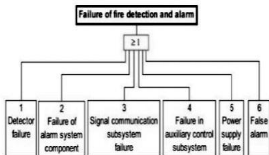
Fault tree of fire detection and alarming system divided into six subunits by cause of failure.
