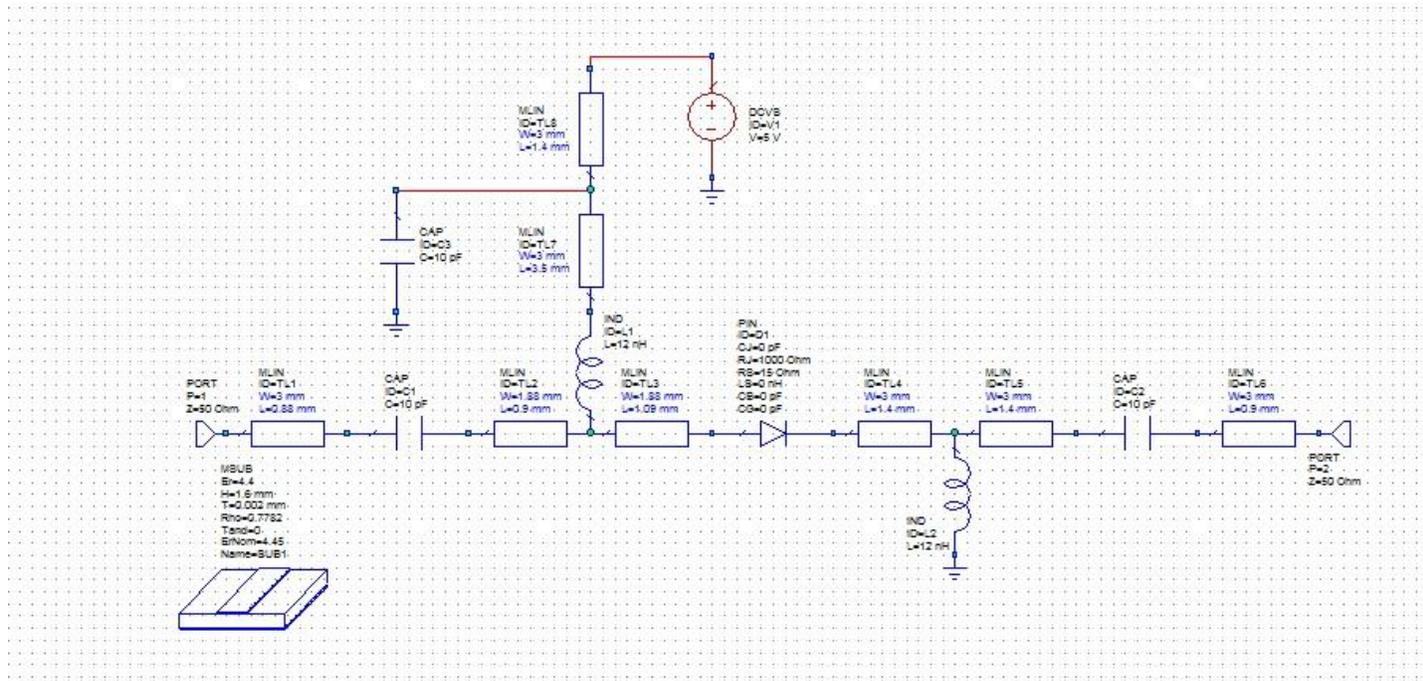
PIN diode circuit
