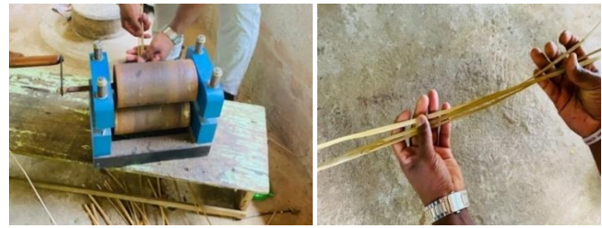
Figure 04: The machine currently used for processing pan and the appearance of the pan plant after processing Source: Field Observations, (2026)
