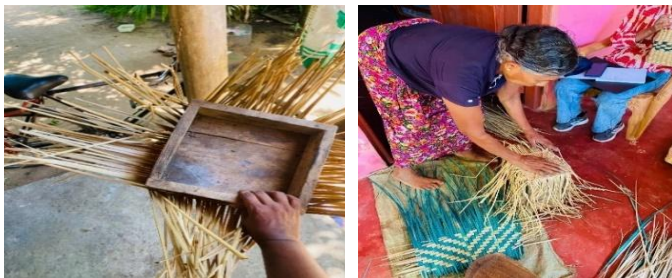
Figure 12: Use of Wooden Moulds for Producing Pan based Products
