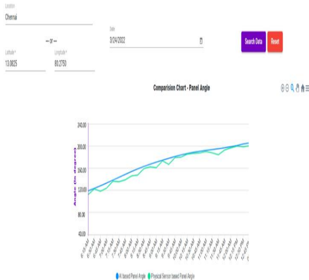
Fig5. Solar Tracker Simulation v/s Sensor based tracker
