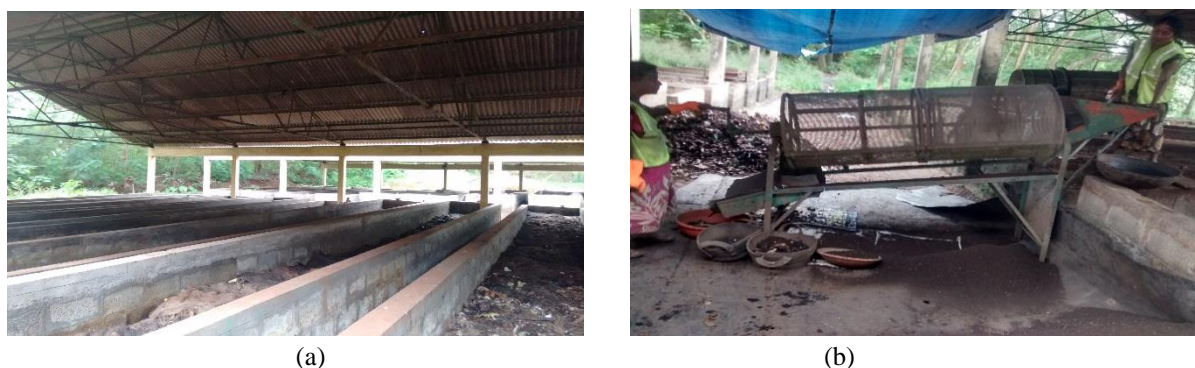
Figure 5: Solid Waste Collection by Vehicles a) Vermi Composting at Mangaluru City Corporation b) Screening of Vermi-Compost at Mangaluru City Corporation
