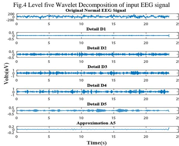
Fig. 5 Wavelet Decomposition of sample EEG epoch of Set A
