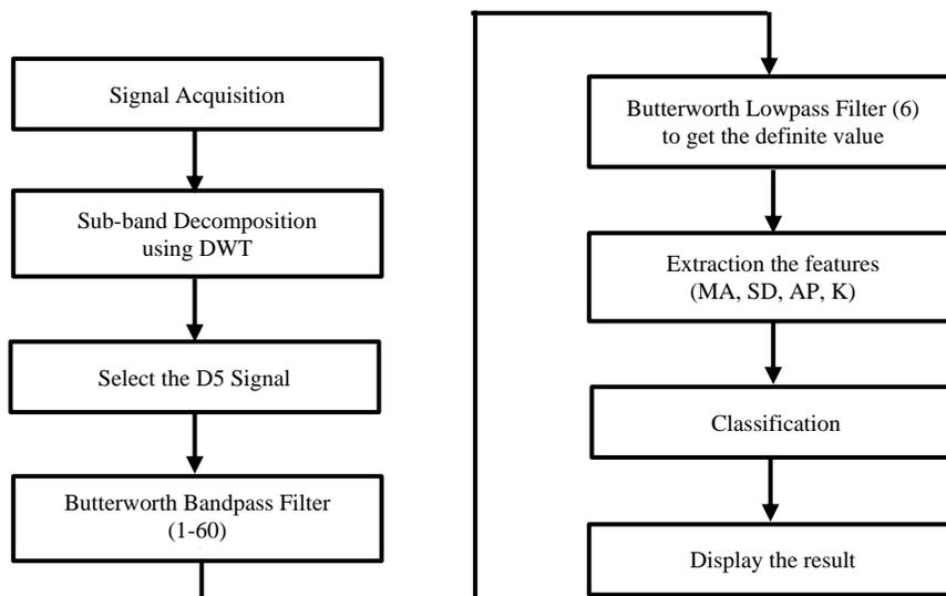
Fig. 2 Flow chart of the overall system
