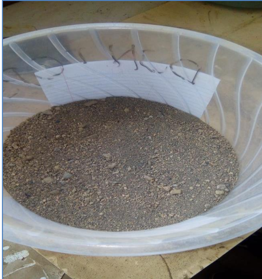
Plate 4 : Mai Mahiu Fine Aggregate without Silt and Fine Dust
