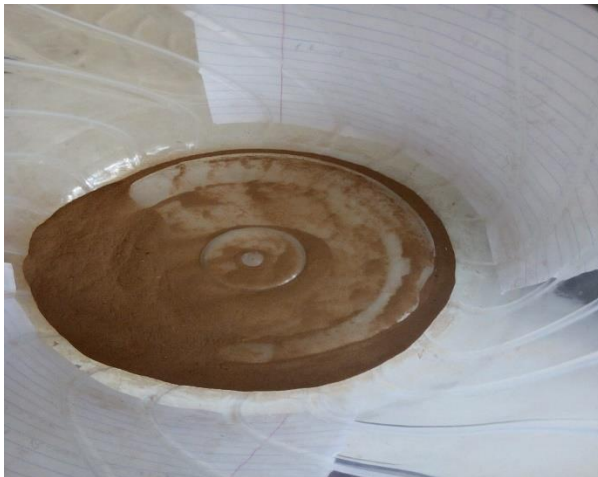
Plate 3 : Silt and Fine Dust Extracted from River Sand
