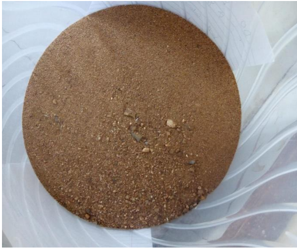
Plate 2 : River Sand without Silt and Fine Dust
