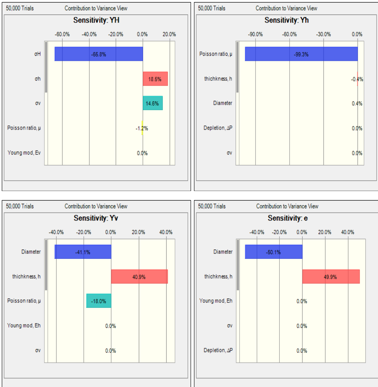
Fig AA: Sensitivity of aspect ratio ( e ), vertical stress path parameter ( \gamma_v ), and horizontal stress path parameters ( \gamma_h and \gamma_H ).
