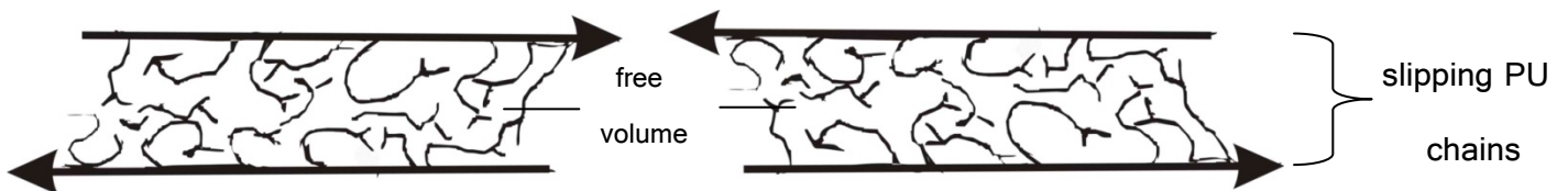
Fig. 3: Schematic arrangement of reactive plasticizer molecules in PU matrix.
