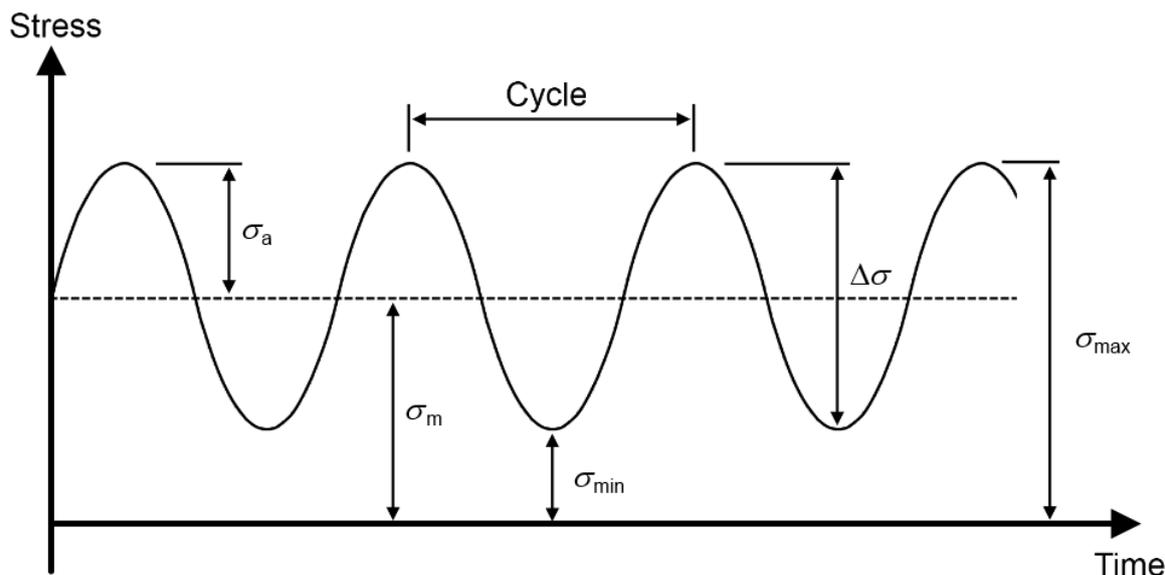
The stress varies between a *maximum stress*,  $\sigma_{max}$ , and a *minimum stress*,  $\sigma_{min}$ , during a load cycle. In the field of fatigue, the variation in stress is often defined using the *stress amplitude*,  $\sigma_a$ , and the mean stress,  $\sigma_m$ . Further, variables defining the *stress range*,  $\Delta\sigma$ , and the *R-value* are frequently used to describe a stress cycle. The relation between the different fatigue stress variables is
