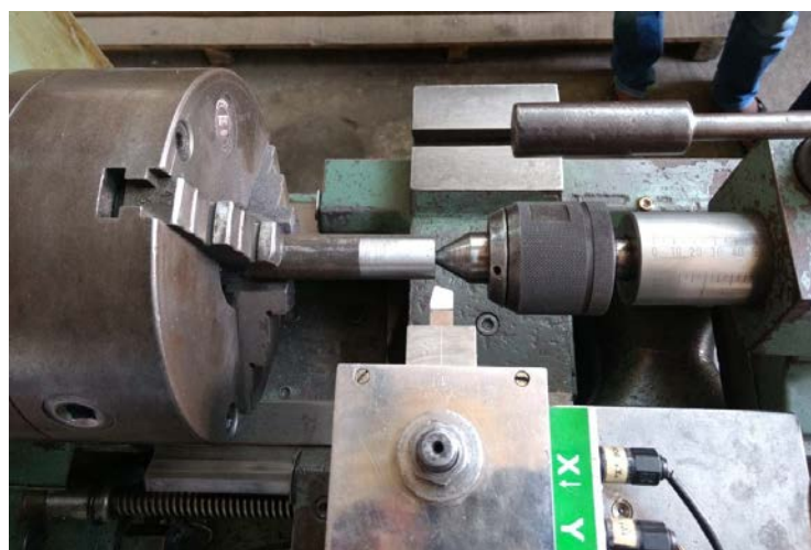
Figure (7): work piece and tool placed in setup along with dynamometre
