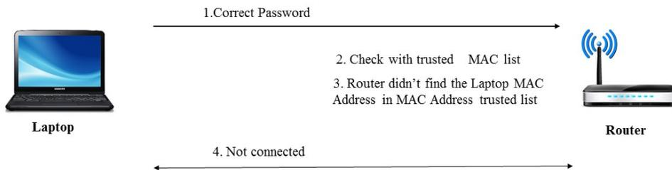
Figure 2: Methodology Overview Diagram (Failed login)
