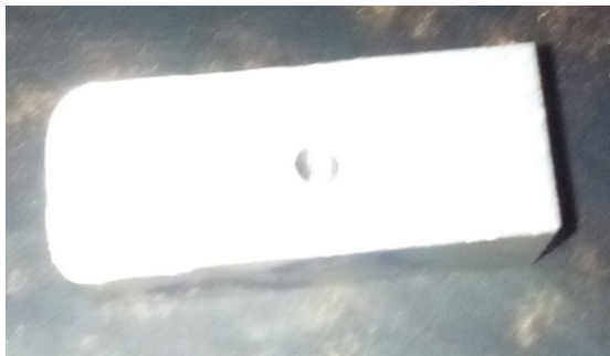
Figure.20 Hardness test specimen Sample 2 - (Aluminium 94%, E-glass fibre 3%, Fly ash 3%)
