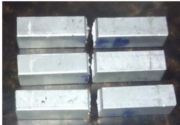
Figure. 24 Impact charpy test specimen Sample 1 - (Aluminium 97%, E-glass fibre 3%)
