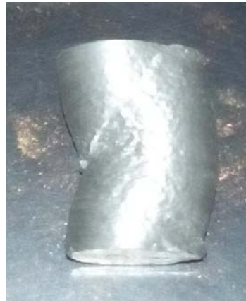
Figure.14 Compressive test specimen Sample 1 - (Aluminium 97%, E-glass fiber 3%)
