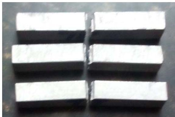
Figure.25 Impact charpy test specimen Sample 2 - (Aluminium 94%, E-glass fibre 3%, Fly ash 3%)
