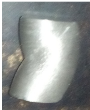
Figure.16 Compressive test specimen Sample 3 - (Aluminium 91%, E-glass fiber 3%, Fly ash 6%)
