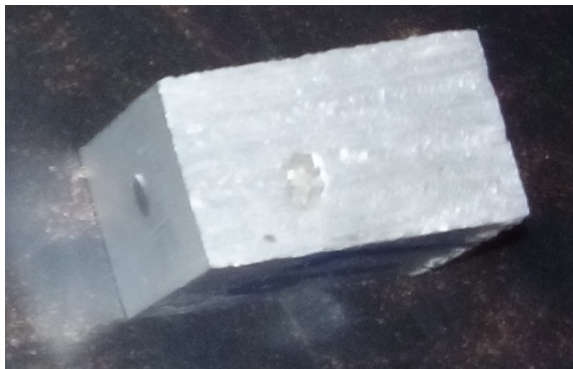
Figure.19 Hardness test specimen Sample 1 - (Aluminium 97%, E-glass fibre 3%)
