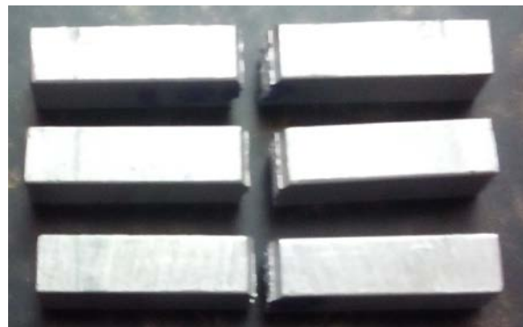
Figure. 27 Impact Charpy test specimen Sample 4 - (Aluminium 88%, E-glass fibre 3%, Fly ash 9%)
