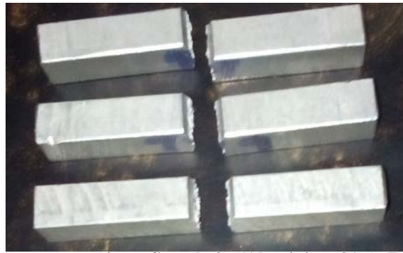
Figure.26 Impact Charpy test specimen Sample 3 - (Aluminium 91%, E-glass fibre 3%, Fly ash 6%)
