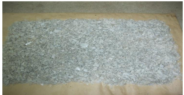
Fig. 1 b: Appearance of LDPE flakes
