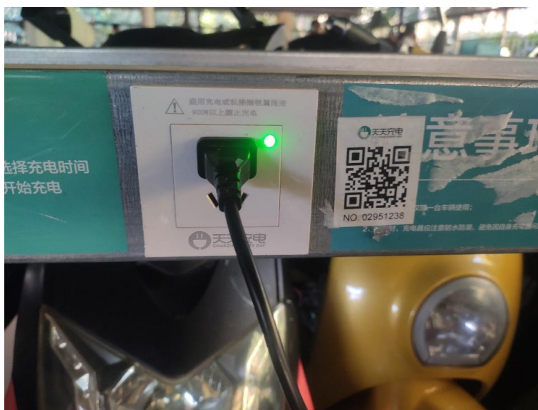
Figure 11: Existing campus charging outlet with a permanently displayed QR code, illustrating the static-code threat scenario
