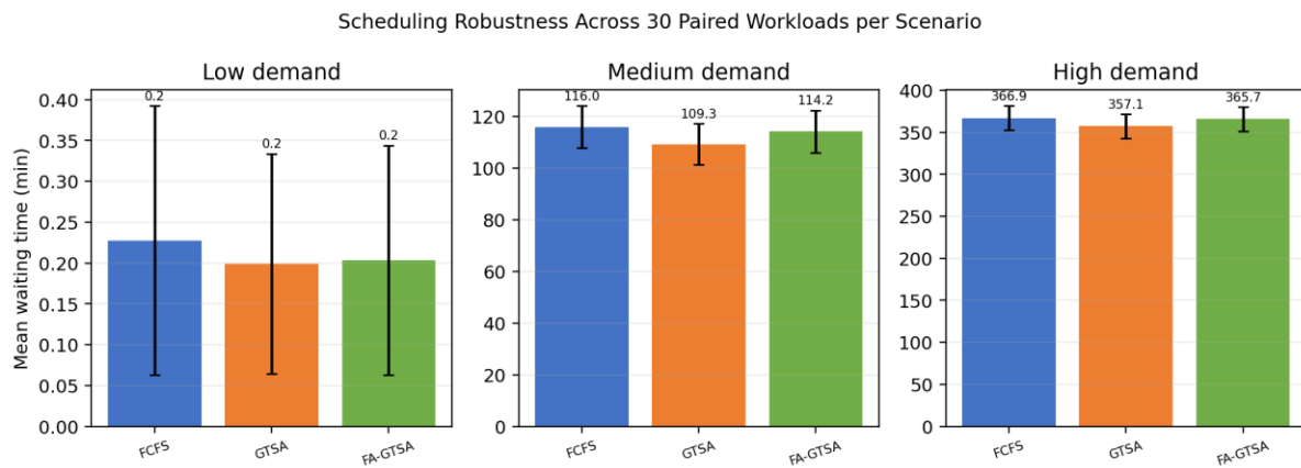
Figure 20: Mean-wait robustness across low, medium, and high synthetic demand; error bars show 95% confidence intervals
