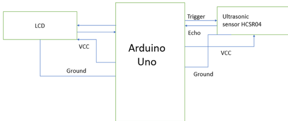
Figure 4: Functional block diagram - Arduino Uno interfaces the HC-SR04 sensing input, local display, and controller connections
