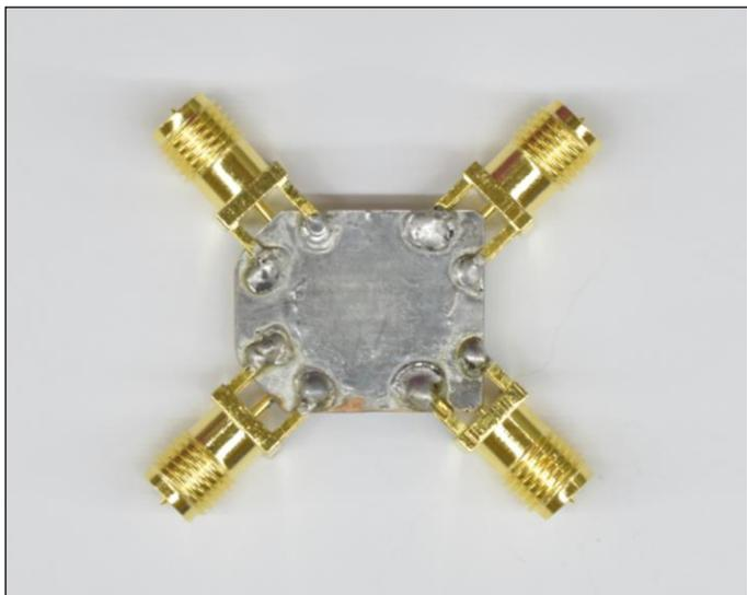
Fig (13): Back side of the module of the lumped-distributed hybrid ring coupler v2
