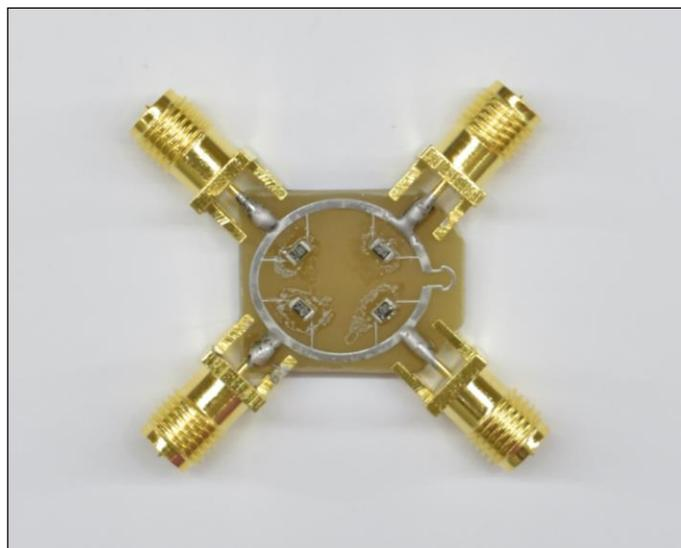
Fig (12): Front side of the module of the lumped-distributed hybrid ring coupler v2
