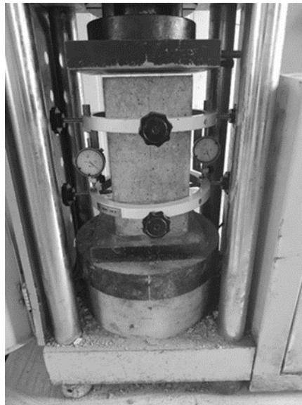
Figure 4. Modulus of Elasticity Testing Equipment undertaken at the Kenya Expressway Project, Nairobi.
