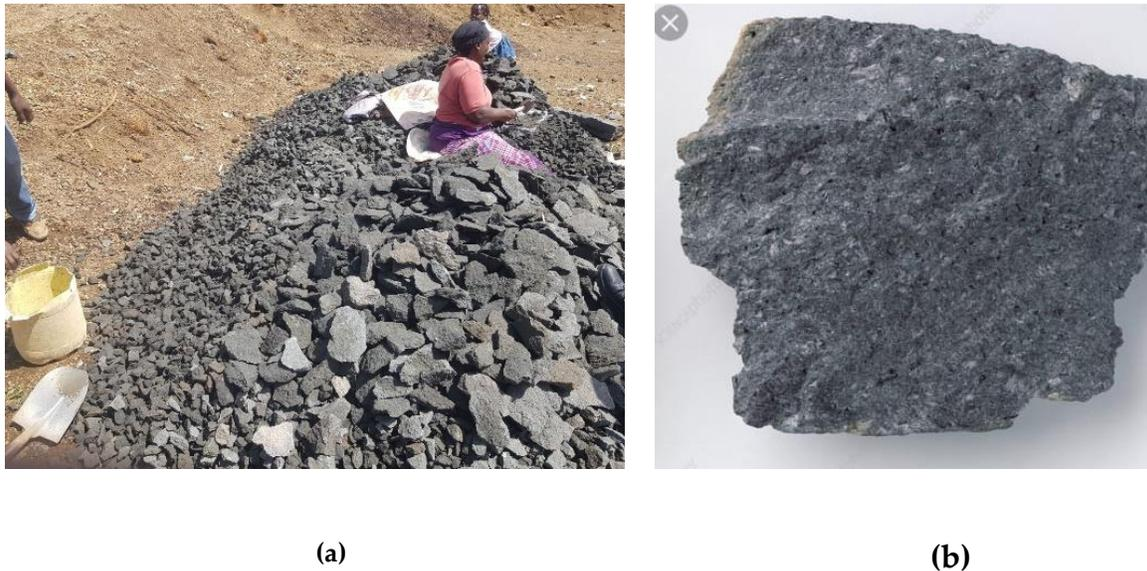
Figure 6 (a) Picture of the Tuff Aggregate sample collected from Nakuru in Bahati Area (0.1671° S, 36.1287° E). (b) Close-up View of the Tuff Aggregate described as Trachyte.
