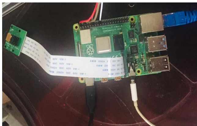
Figure 1: Camera module connection to Raspberry pi
