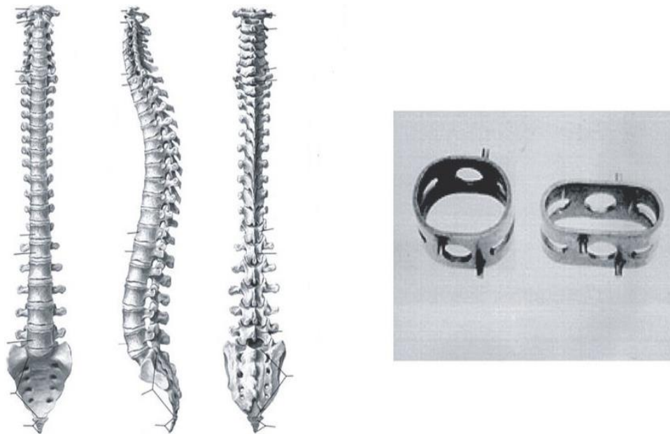
Figure 3: b. Spinal Vertebrae Spacer in the martensitic state (left) and in the original shape (right) [11].
