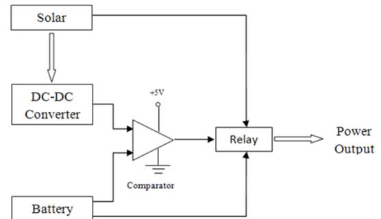
Figure 1 Block Diagram of Hybrid Power Supply
