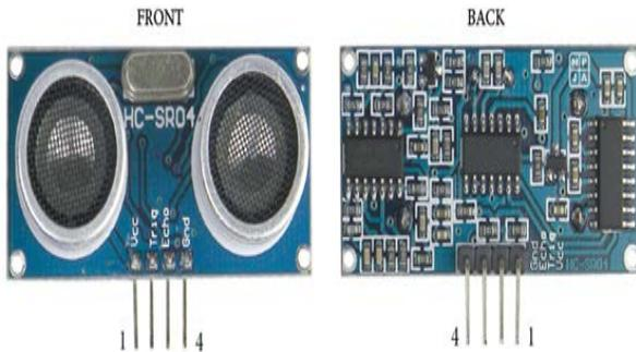
Figure 5 Front and Back View of HC-SR04 Ultrasonic Module
