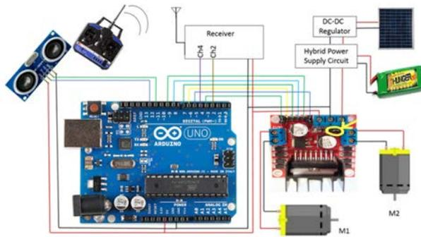
Figure 8 The whole circuit diagram of solar car
