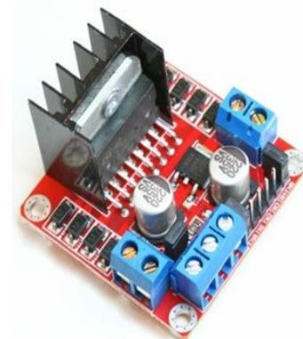
Figure 7 L298N Motor Driver Module
