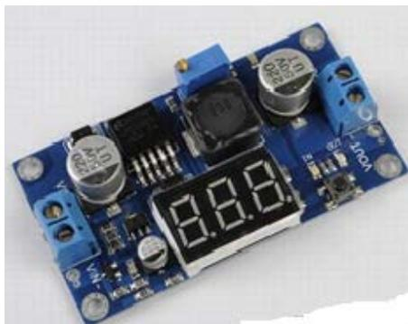
Figure 2 DC-DC Converter Circuit Board
