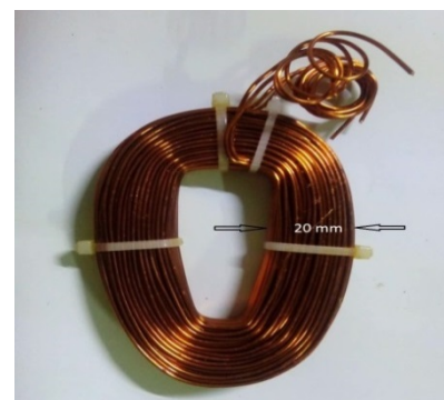
Fig.3 Two Strings 18 SWG wire 70turns winding
