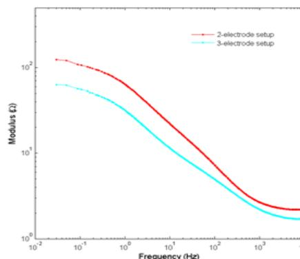
Figure 7. Modulus of the impedance of zinc in 1 M NaCl after 15 h immersion using the two-electrode and three-electrode setups.
