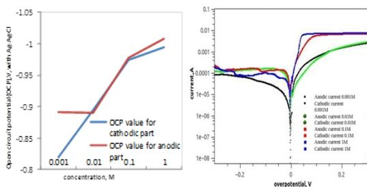
Figure 1. (a) Open circuit potentials for the different concentrations. (b) Cathodic and anodic polarization curves of zinc in different sodium chloride solutions with the three-electrode setup.
