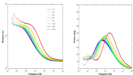
Figure 3. Bode plots of the impedance of zinc in 0.01 M NaCl with the two-electrode cell during 24 h immersion. (a) Modulus. (b) Phase angle.
