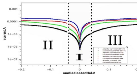
Figure 2. Cathodic and anodic currents for zinc in different sodium chloride solutions with the zinc-zinc two-electrode setup.
