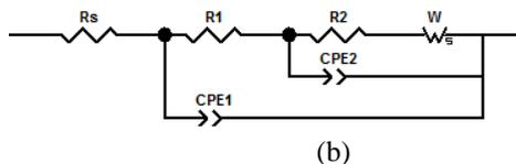
Figure 6. Electrical equivalent circuits used to model the impedance experiments.
