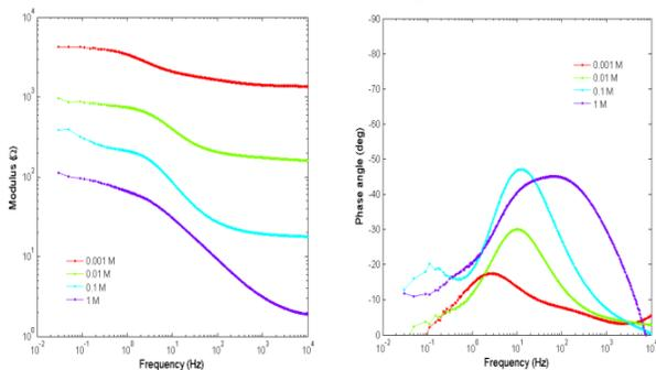
Figure 4. Bode plots of the impedance of zinc in different concentrations of NaCl with the two-electrode cell after 2 h immersion. (a) Modulus. (b) Phase angle.
