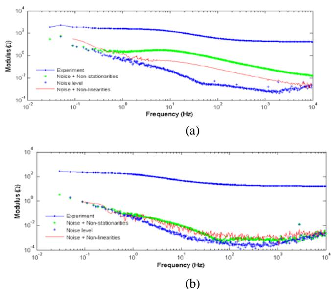
Figure 5. Analysis of the linearity and the stationarity of the impedance measurements of zinc in 0.01 M NaCl with the two-electrode cell: (a) after 2 h; (b) after 12 h.
