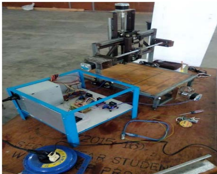
Figure 10. Final Assembly Of Machine Frame, Stepper Motor And Motor Control Circuit
