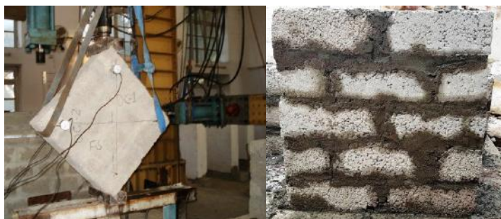
Figure 8: Diagonal Shear Strength Test
