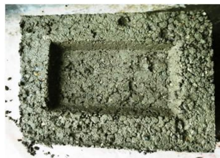
Figure 4: Frog Concrete Block Specimen
