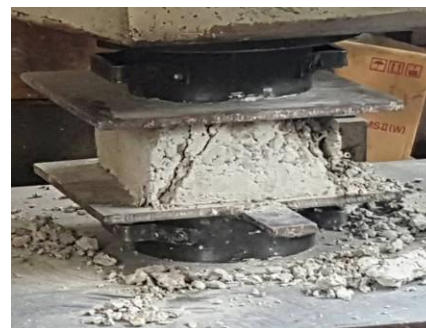
Figure 5: Unit Compressive Strength Test
