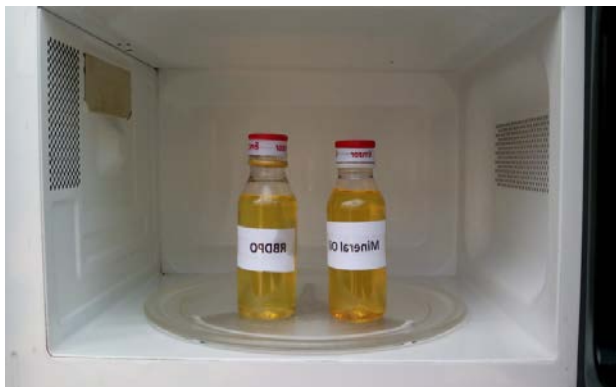
Figure 1: Photo of oil samples in the oven for accelerated aging process
