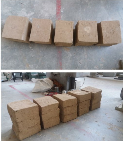
Fig3: Prepared specimens for compression test
