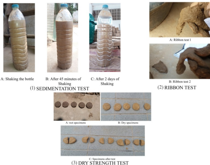
Fig1: Site test to identify the soil.
