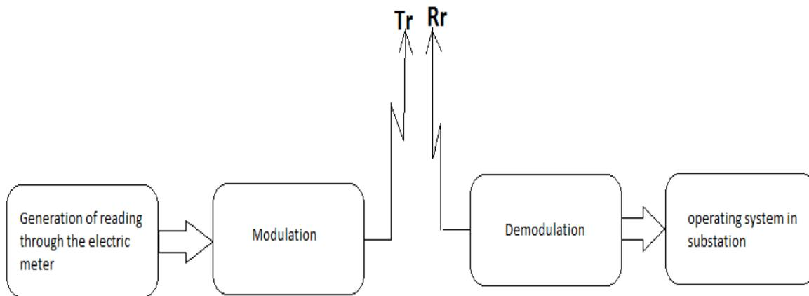
The transmitter uses mobile communication networking architecture to transmit the signal to substation and only one man require to operate these in substation.
