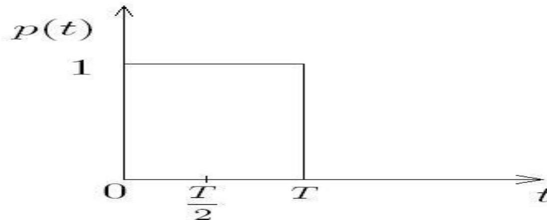
(a) the spectrum of a rectangular pulse is infinite in extent. Correspondingly, its frequency content is also infinite. But a wireless channel is bandlimited, means it would introduce signal distortion to such type of pulses,
