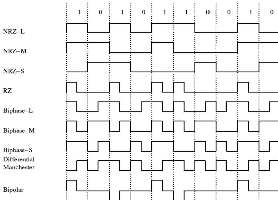
7. Biphas-S: There is always a transition in the beginning of a bit interval. 0 forces a transition in the middle of the bit while 1 does nothing.
